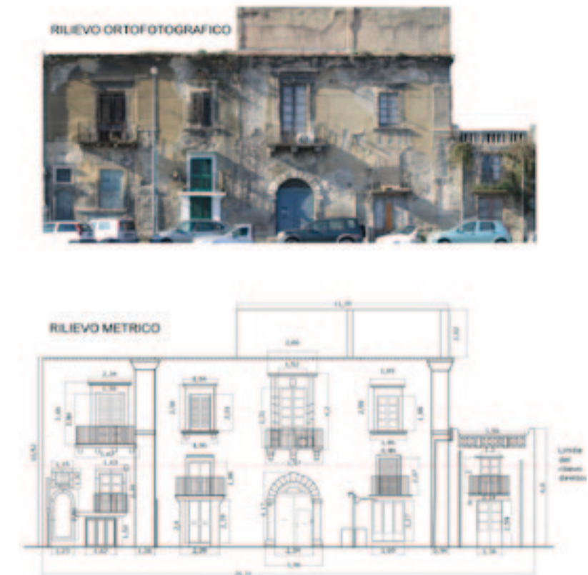
Fig. 8 – Metric and orthophotos survey of East elevation of the Formento building in Messina. Processed during the course of Architectural Restoration (AA.2008-09 – prof. Fabio Todesco) Degree in Civil Engineering, University of Messina. Students: Alessandra Cernaro, Carmela Malarbi, Roberta Parisi.
